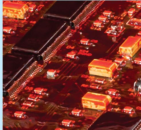
VFD lifespan is extended by a varnish with protection against dust, humidity, high temperatures and some chemicals. This process called **Conformal Coating** (tropicalization) is standard for all CFW, SSW, SCA and MW500 lines, classified as 3C2 according to IEC 60721-3-3.
