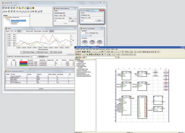
Software application of WEG for VFD, servo drives and soft-starters can be downloaded on the website for free. SuperDrives G2 is a powerful tool permitting parameter setting, command and monitoring simulating an oscilloscope. Also the WLP allows the creation/edition of applications for the SoftPLC being a smart and simple way to make your drive or soft-starter, motor and application work together. WPS is all-in one software, SuperDrive G2 + WLP.
