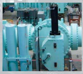
This butterfly valve is controlled by a Ø10" actuator equipped with a Ø3.5" high-strength stainless steel piston rod along with electronic feedback and banked accumulators
