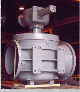
This  $\emptyset$ 24" cone valve (above) is controlled by a  $\emptyset$ 6" x 14" stroke actuator with a 2" stroke adjustment, stainless steel rod and special protective paint.
